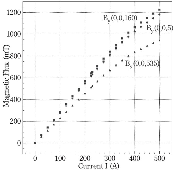
Fig.3. Measured magnetic fluxes  $B_y$  at three points with different coil currents. The deep gray circle, rectangle, and triangle markers show those at  $(0,0,0)$ , at  $(0,0,160)$ , and at  $(0,0,535)$ , respectively, where the coil currents are set in the decreasing direction. The light gray circle, rectangle, and triangle ones show those at  $(0,0,0)$ , at  $(0,0,160)$ , and at  $(0,0,535)$ , respectively, where the coil currents are set in the increasing direction.
