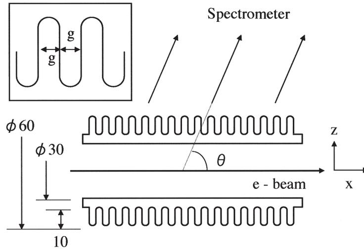
Fig.1. Schematic layout of the experiment. The electron orbit is shown by the thick solid line. The emission angle  $\theta$  was measured from the  $x$  direction. The inset shows the shape of groove.
