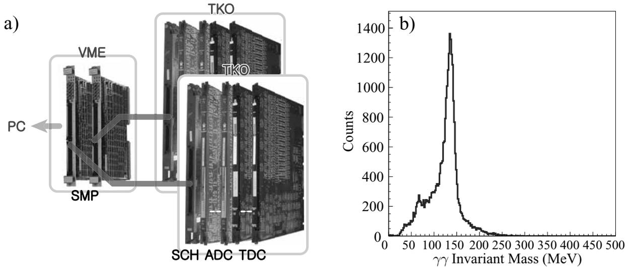
Fig.3. a) Dataflow of the data acquisition system for SCISSORS III. The digitized data of energies and timings are collected from ADC's and TDC's in a TKO system through SCH and SMP modules. b) The  $\gamma\gamma$  invariant mass distribution measured with SCISSORS III. The  $\pi^0$  peak is clearly observed.
