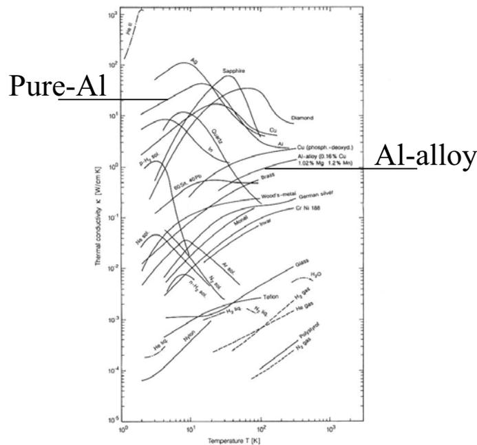
Fig.2. Thermal conductivities as a function of temperature for some materials. Pure-aluminium has high thermal conductivity at our operation temperature  $\sim 10$  K.
