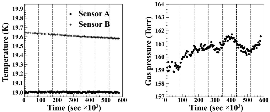
Fig.7. Trends of the temperatures and the gas pressure of the target cell with liquid  $D_2$  in a week. The vertical broken lines are drawn every 24 hours. Each value is stable for a long time.
